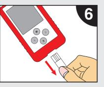
5. The meter will beep and count 25 seconds to show the result in per mill (‰) 6.Remove the strip and discard it accordingly
