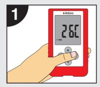
1.Check temperature, that it's in the operating range. If there's a rapid >10°C (>18°F) change, wait for the system to stabilize for 10 minutes
