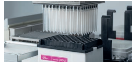
Multiple Channel Arm picking up 96 500 \mu\text{L} disposable tips
