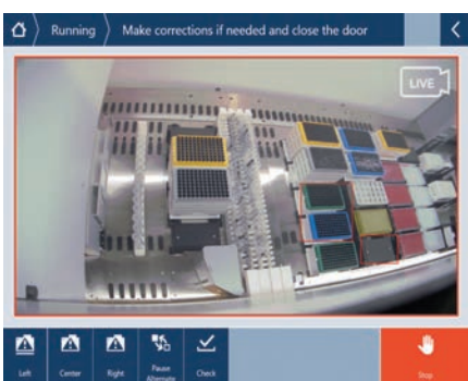
DeckCheck highlights differences to the expected worktable
