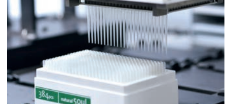
Multiple Channel Arm picking up one row of 24 50 \mu\text{L} tips
